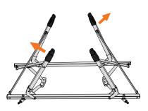
2. Place the frame on the floor, with the legs facing upwards, pull the legs outwards until the frame is fully open.
