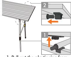
1. Pull out the plastic ring from the end of fixing tube.
