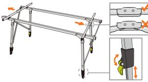
3. Release the trigger before adjusting the length of the table leg. After adjusting the length of the table leg, please lock the trigger to ensure the table stability.
