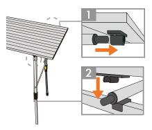
4. Clip the plastic ring into the head of fixing tube.
